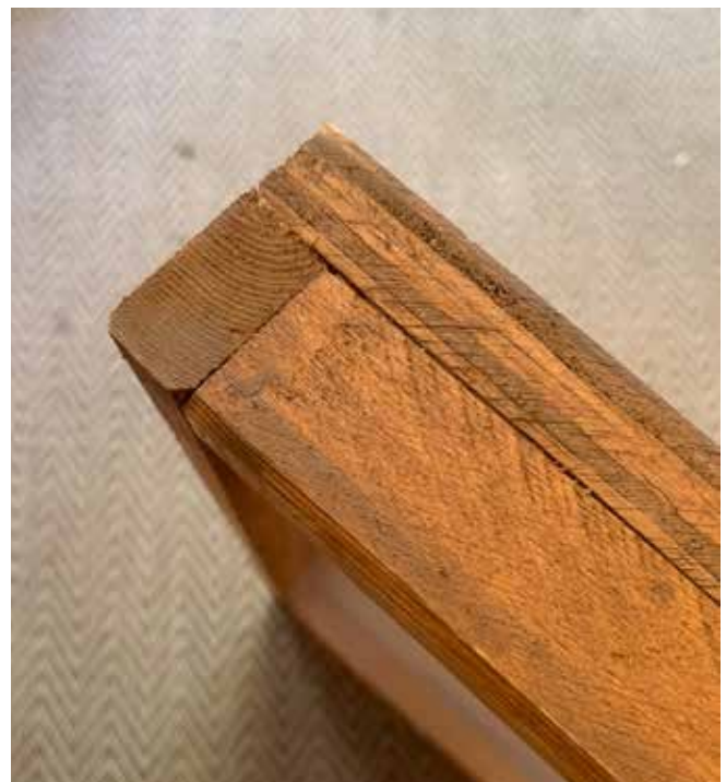
If adding sides, a nail gun works best to tightly nail the corners together.
