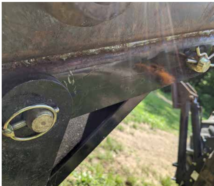
I found that a lynchpin (the snap-ring style to the left) hangs on better than the hairpin style to the right.
