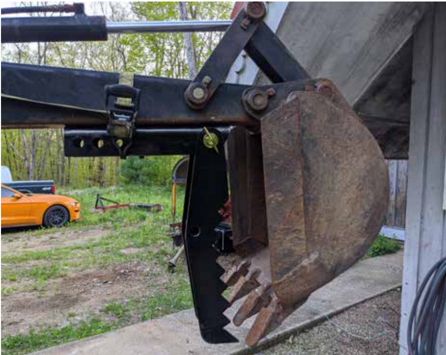
Be sure to measure your bucket while it sits at a 90-degree position, like pictured, when sizing a thumb for your machine. Also, be sure to test fit your thumb before permanently attaching it.
