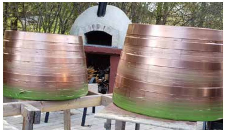
Top: Because spray paint will be used to paint the metal bands, a full roll of painter tape was placed over the stained wood and the metal bands were sanded down again one last time.
