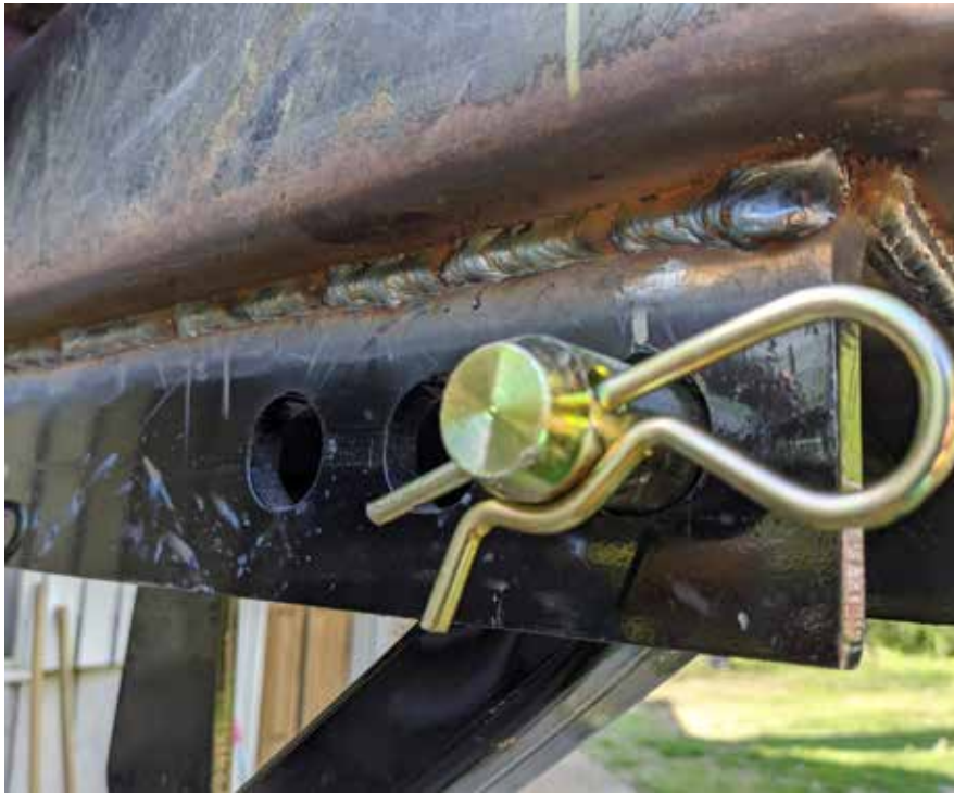
Not my finest welding, but my backhoe thumb is stuck on with no signs of giving up.
